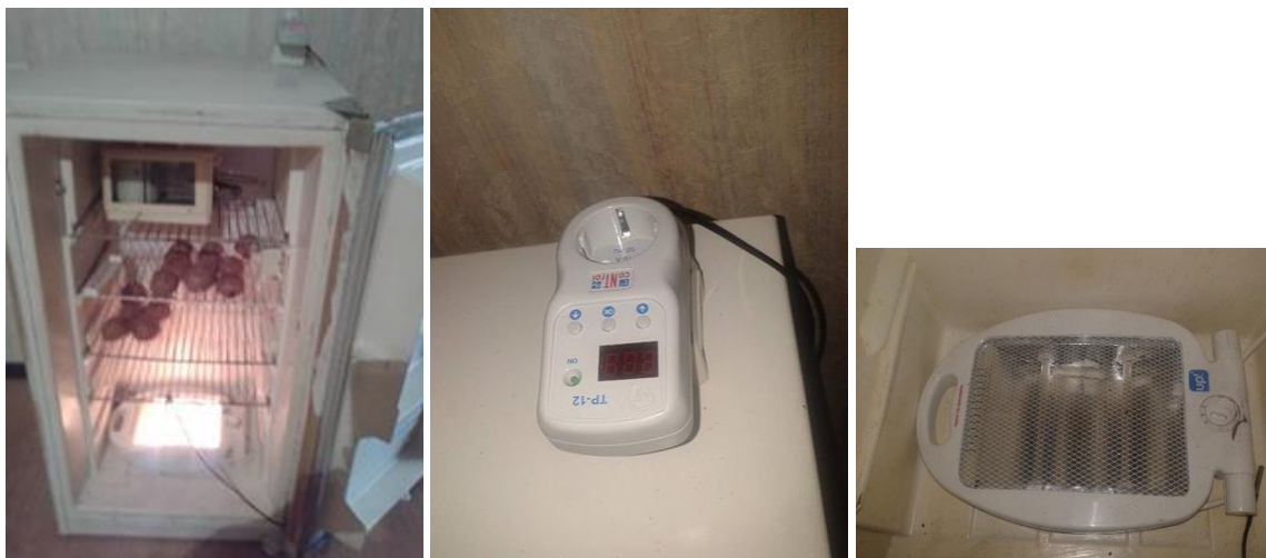
Fig. 4. Thermal cabinet, thermal relay and heater
